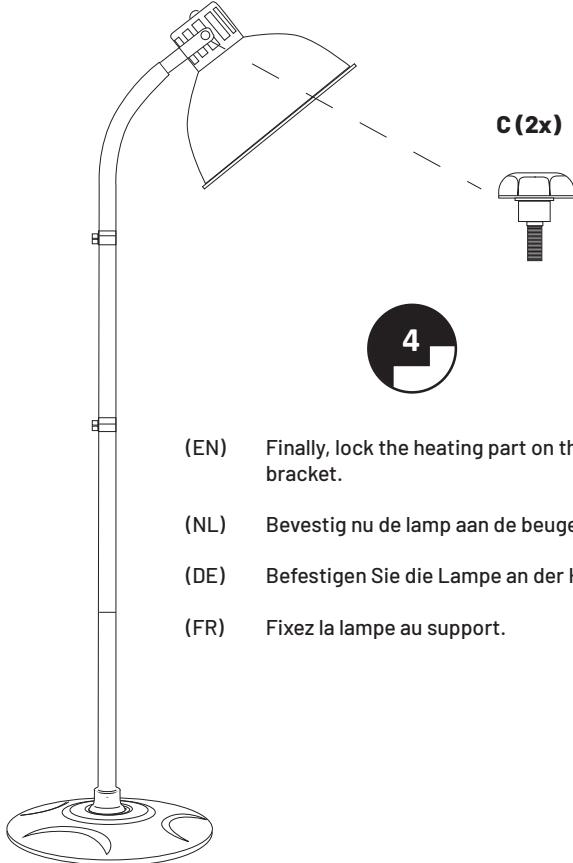
(EN) Finally, lock the heating part on the adjustable bracket.
