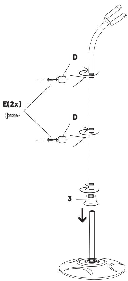
(EN) Place (D) on bottom tube and screw the next tube clockwise into the bottom tube and tighten with (E). Repeat with top tube.
