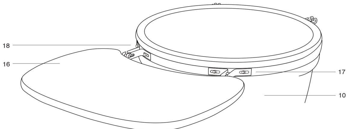
**STEP 16 -** Insert the 2x table hinge into each of the table brackets (20 & 21).
