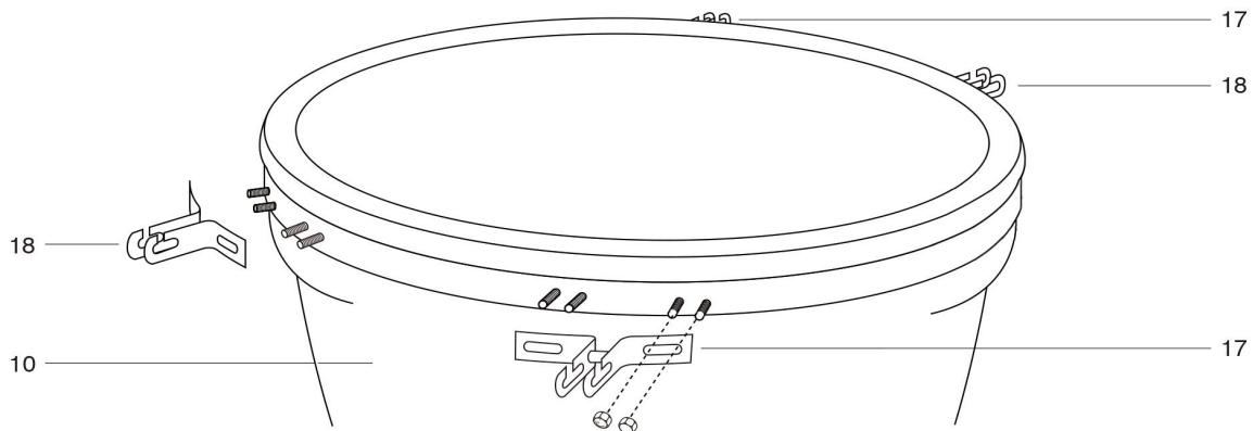
**STEP 14 -** Attach the 2x table brackets (20) to the Kamado Grill (12) using the 4x pre-attached bolts and dome headed nuts per bracket. Please note the position shown in the above diagram
