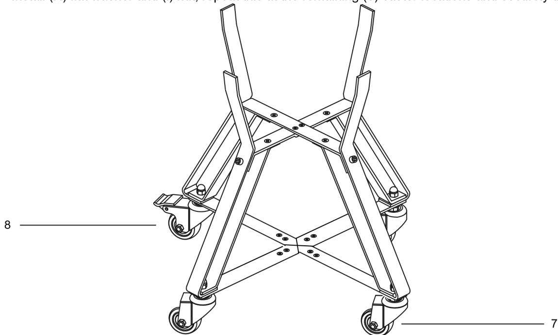
**STEP 4 -** As picture, put wheels 7 in front, and wheels with brake at the back.
