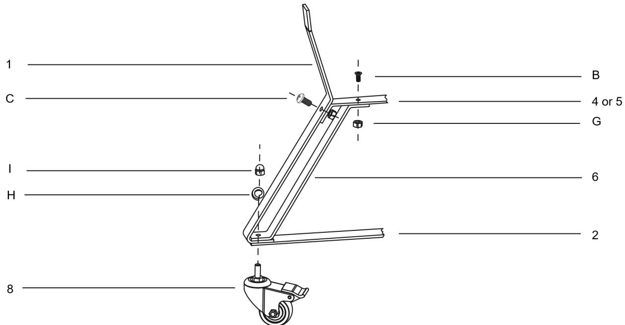
**STEP 2 -** (Joining the two halves assembled in step 1) Stand the section 1 upright, and place the upper cross braces (4&5) close to section 1. Inserting truss head screw C through the hole of section 1 and section 4&5 and install G nut and tighten securely.
