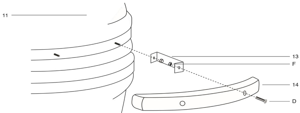
**STEP 12** - To attach the handle (14) to the lid of the Kamado Grill (11) start by attaching 2x handle brackets (13) using the 2x pre-attached bolts and dome headed nuts. Attach the handle (14) to the brackets (13) using 2x bolts (D) and nuts (F)
