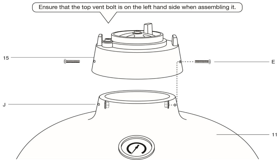
**STEP 13** - To attach the top vent (15) to the Kamado Grill (11) place it on top and align both the bolt holes. Secure using 2x bolts (E) and nuts (J). Ensure that the top vent bolt is on the left hand side when assembling it.
